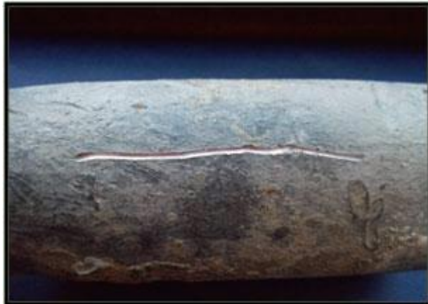
A lead pipe can be easily scratched with a key. (2)
